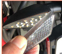
REPLACING THE LENS
