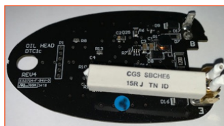
WEISER UNIT WITH RESISTOR FITTED
